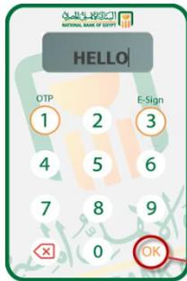
After you switch on the hard token as illustrated in section two of this manual, press and hold OK for two seconds.
